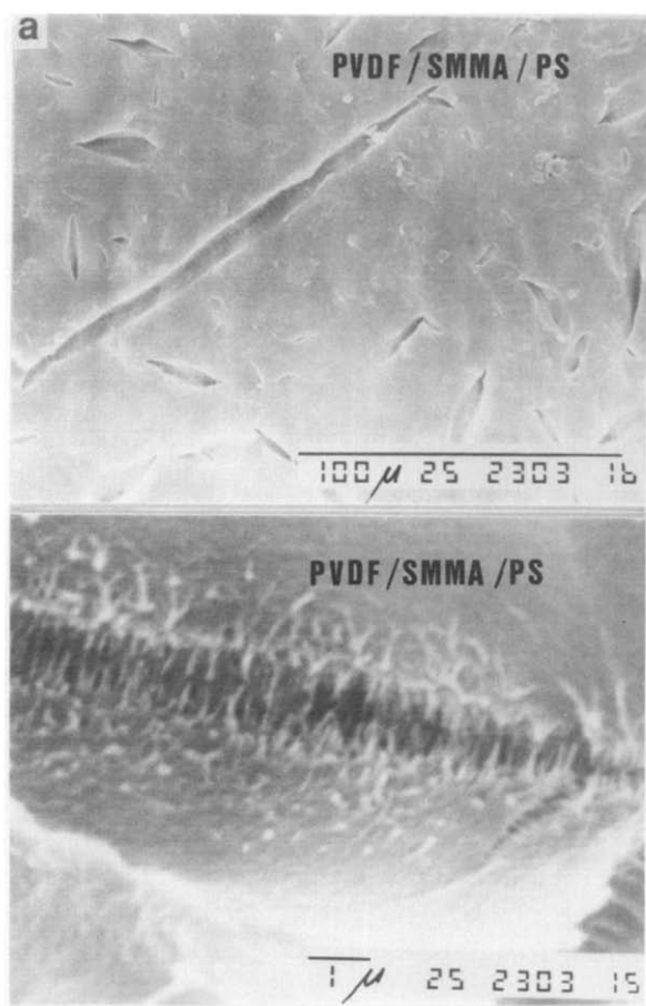
Figure 8 SEM of PVDF surfaces pressed against (a) SMMA copolymer with 5% styrene and (b) PMMA/PS blend with 10% PS at 185°C and 300 atm
