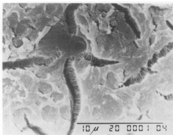
Figure 6 SEM of PVDF surfaces pressed against PMMA at 185°C and 0.1 atm after extraction with chloroform
